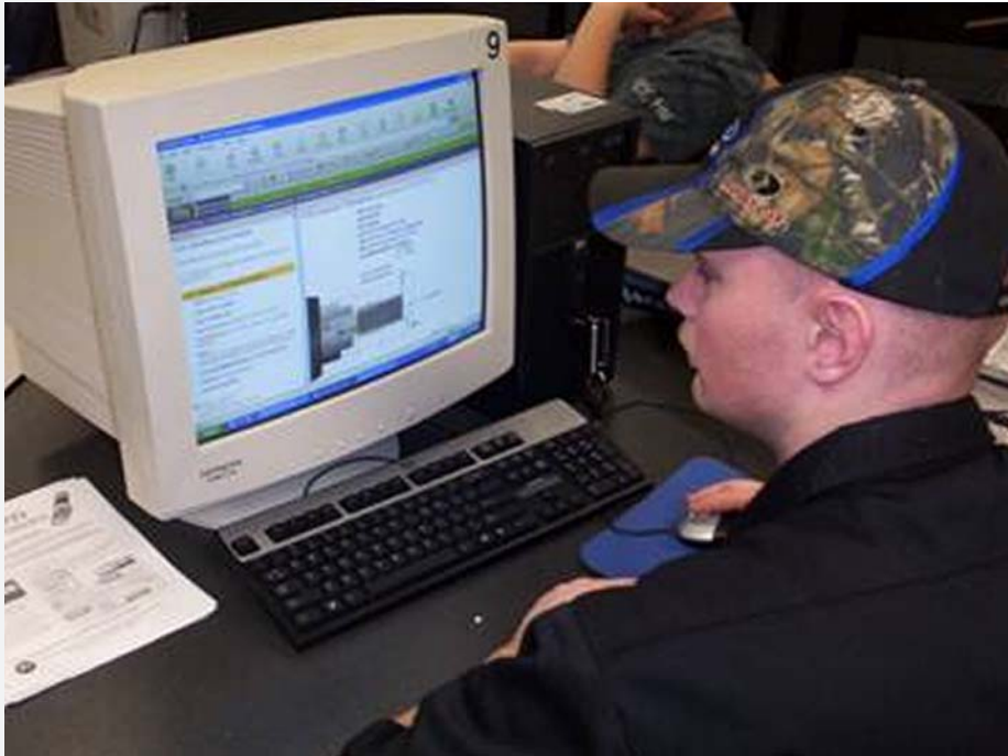
Students are required to prove-out setup and M&G code programming skills with virtual CNC controls and 3D machines, interactive curriculum and assessments before doing the real thing.
