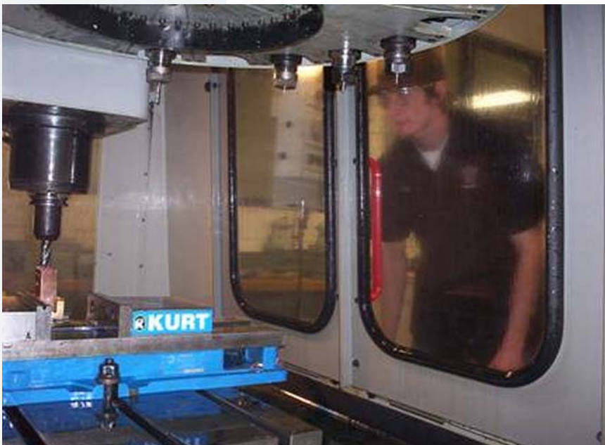
A student inputs tool offsets, prior to running a part program that was written and visualized with VTE-CNC virtual control panels and simulate 3D machines.
